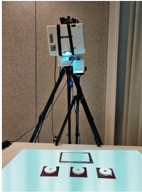
Figure 4.1: The hardware setup of the system used to create the MR framework. Lashing straps are used to firmly attach the projector to the tripod. The camera is set up on a separate tripod. This allows for easy adjustment of the hardware’s position and height when needed.
